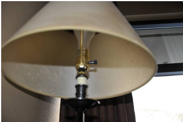
16 Lamp switch requires tight pinching, grasping, twisting of the wrist to operate
